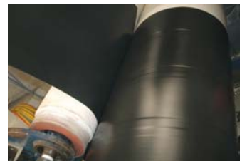
3-Layer polyethylene coating (3LPE)
