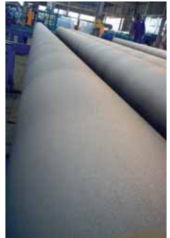
Shot Blasted Pipe
