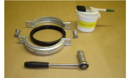
2. Ensure the pipe ends are within tolerance and free from score marks, indentations and excessive build-up of coating materials. Apply a thin uniform coat of a suitable non-petroleum based lubricant on both pipe ends around the entire circumference.
